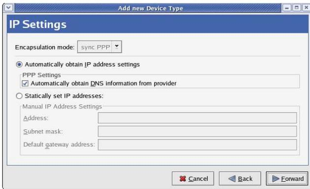
**Fig. Filling in the IP Settings**
