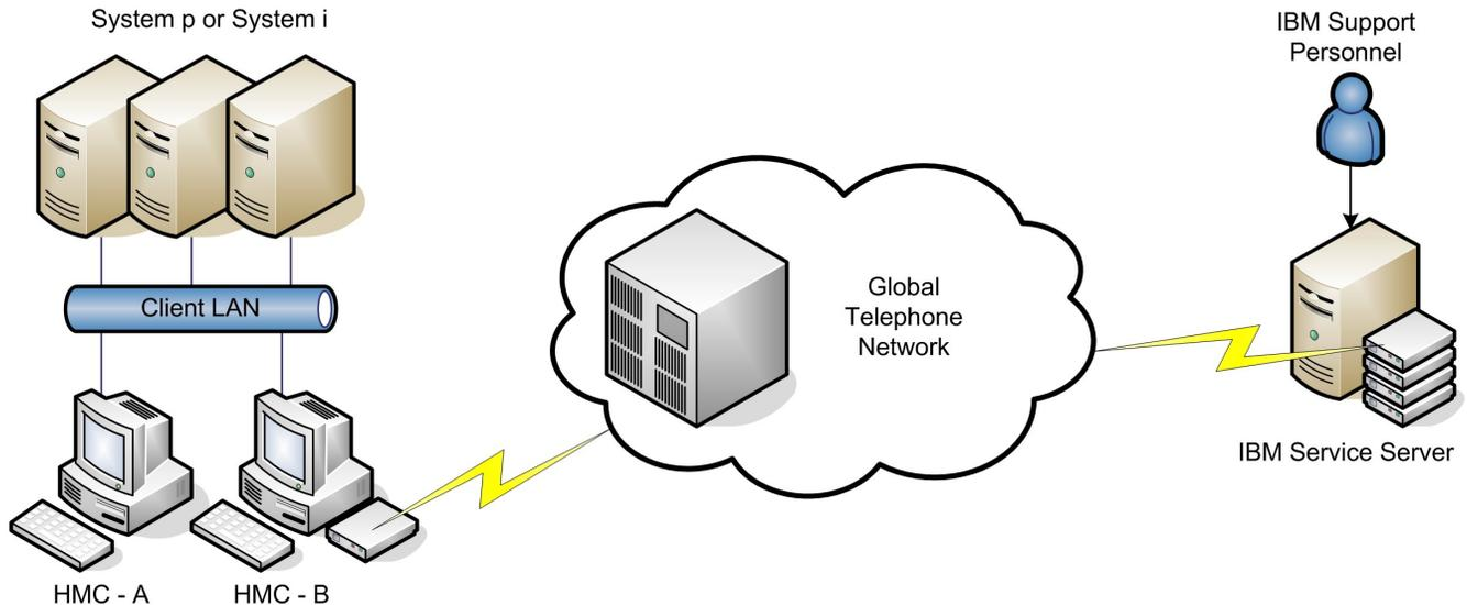
For remote service over a modem, the modem must be set up to accept incoming phone calls. An IBM representative then logs into a special server and uses that to dial directly into the client's modem. After the modem answers, a PPP session is initiated, and the IBM representative must authenticate using credentials based on the value the client entered into the **PPP address** field on the Customize Inbound Connectivity panel.
