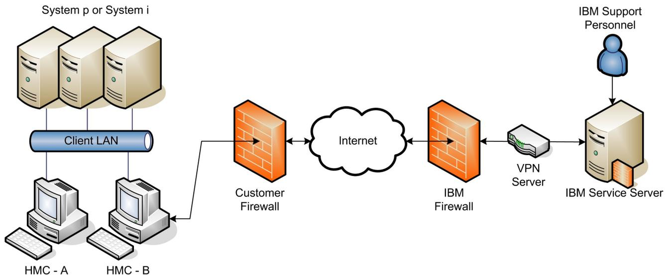
A remote service VPN session can be initiated over a modem, Internet VPN, or a pass-through i5/OS partition. At least one of these methods of connectivity must be configured through the Outbound Connectivity panel.
