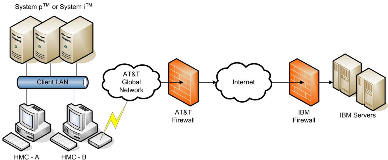
In this scenario the HMC uses one of the configured phone numbers to dial the modem, connecting to the AT&T Global Network. After the modem connects the HMC authenticates itself and establishes a Point-to-Point Protocol (PPP) session between the two modems. Finally, after the PPP session has finished, AT&T allows IP connections through a “Fenced Internet,” which completes the network between the HMC and the IBM servers.
