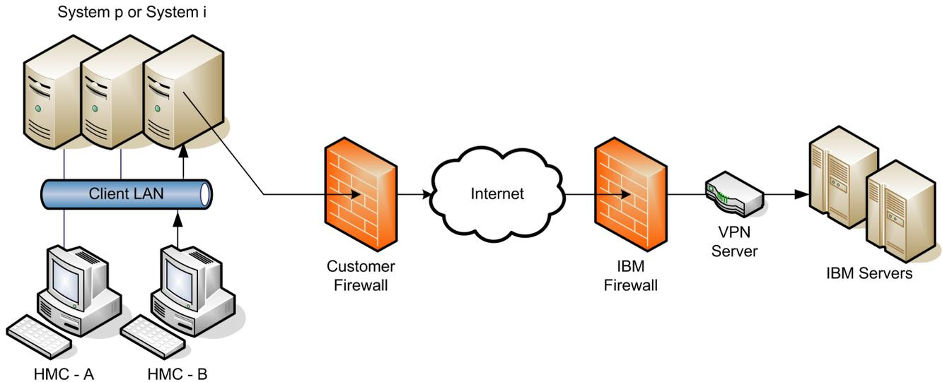
Before the HMC tries to connect to the IBM servers, it first establishes an unencrypted Layer 2 Tunneling Protocol (L2TP) tunnel to the i5/OS partition and requests the creation of an encrypted VPN tunnel between the partition and the IBM VPN server. The HMC initiates this tunnel using a UDP socket. After it is established, all further communications are handled through TCP sockets, which always originate from the HMC.
