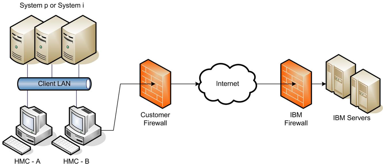
In this setup the HMC connects through the client-provided Internet connection by the default route. For this type of configuration the client can optionally use a second network card to physically separate the local system network from the Internet-enabled network.
