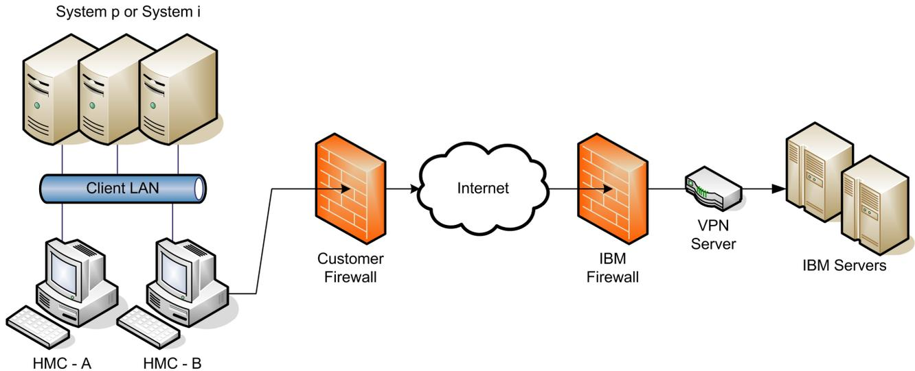
In this setup the HMC connects through the client-provided Internet connection by the default route. For this type of configuration the client can optionally use a second network card to physically separate the local system network from the Internet enabled network.
