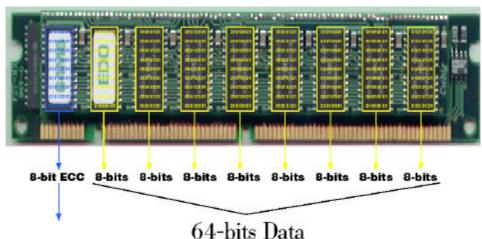
On current high-performance Intel processor-based file servers, these memory chip failures cause a system crash that can result in the permanent loss of several gigabytes of business data! This is a catastrophic failure with no possible data recovery in most file server applications.
