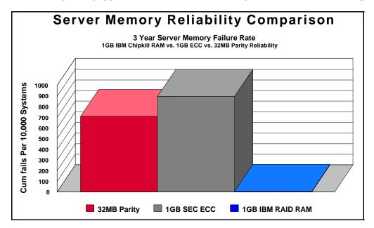
Failure rates for 1GB ECC memory are actually higher than failure rates for 32MB parity memory! The reason is that the number of 64Mbit DRAM modules required to supply 1GB of memory has increased to the point that there is a greater potential for a memory chip failure than there is for a single-bit parity error when using 32MB of parity memory. IBM Chipkill Memory technology reduces the failure rate of IBM Netfinity servers to an incredibly low 6 failures in 10,000 systems for a 3-year lifetime!
