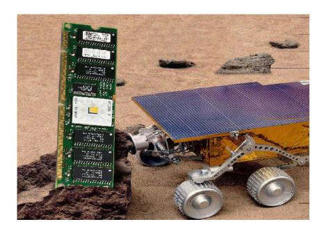
Notice the white RAID chip in the center. This chip performs the ECC calculation for each data access and stores the result in additional DRAM modules on the DIMM. Chipkill technology was used by NASA in the Mars Pathfinder probe. NASA engineers understood that this problem was real and they did not want to invest the billions of dollars to send the Pathfinder probe all the way to Mars only to have the entire mission ruined by a memory chip failure!
