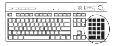
Press the Num Lock key to lock and unlock the numeric key functions:
