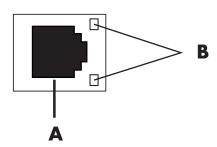
With the PC turned on, check the lights (B) next to the Ethernet connector for status:
