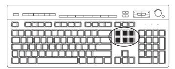
The edit keys are Insert, Home, Page Up, Delete, End, and Page Down. Use these keys to insert and delete text and to quickly move the cursor on your screen. They function differently with some software programs.
