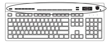
There are special buttons (select models only) at the top of the keyboard. (Some models have some of these special buttons on the left side of the main keys.) These buttons operate a CD or DVD player, control speaker volume, connect you to the Internet, or provide quick access to specific functions.
