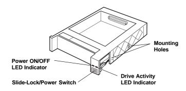
Latch-Lock Model Mobile Rack Docking Case
