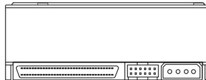
The previous illustration shows the pin positions on the 36.4GB Ultra SCSI 1.6" high disk drive.
