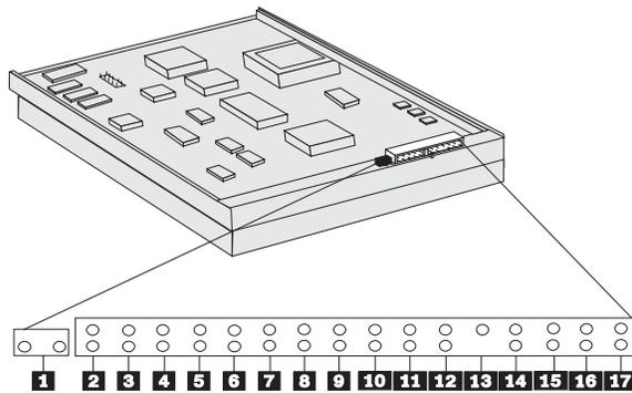
The jumper block on the drive has 16 pin positions (2 through 17). Term Power Enable (1) is located to the left of the jumper block. Refer to the previous illustration.
