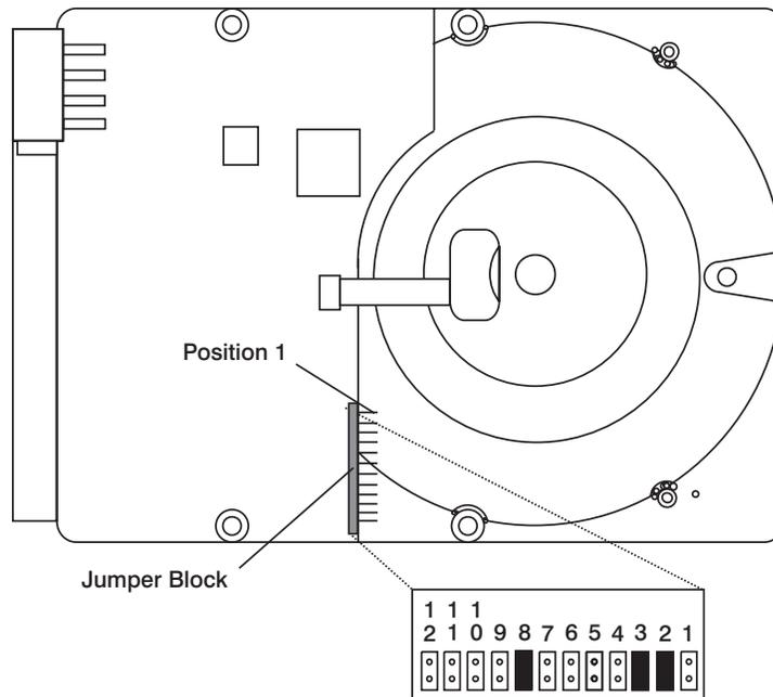
The previous illustration shows the pin positions on the 9.1 and 18.2GB Ultra SCSI disk drives.
