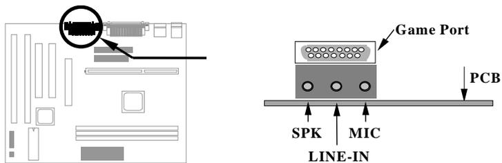
To fully utilize the audio functions, you may connect various peripheral devices that the audio chip supports. The following figure shows the different devices that you can connect.
