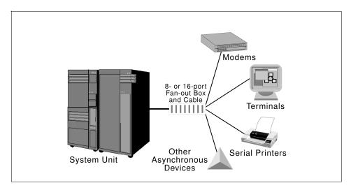
Figure 3-9 Terminal connection to direct-attached asynchronous adapter
