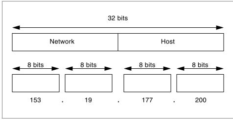
Figure 10-5 IP address format
