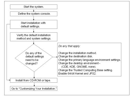
Figure 4-1 shows a flow chart of the steps for installing a system.
