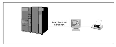
Figure 3-8 Attaching a serial terminal to an RS/6000 system
