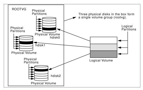
Figure 6-1 Relationship between logical storage components
