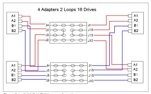
Figure 7-1 7133-D40/T40 loop configuration
