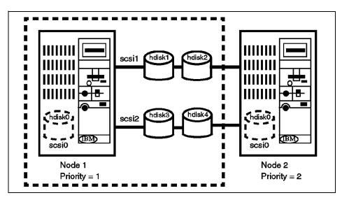
Figure 2-6 Hot-standby configuration
