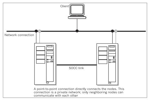
Figure 2-11 Point-to-point connection
