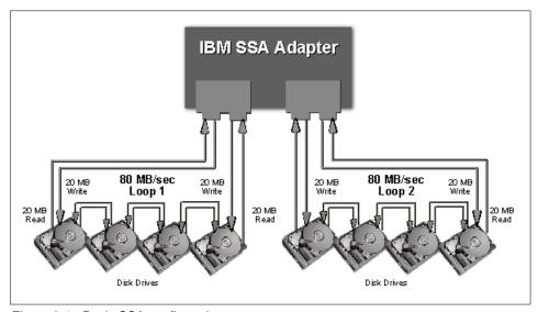
Figure 2-1 Basic SSA configuration
