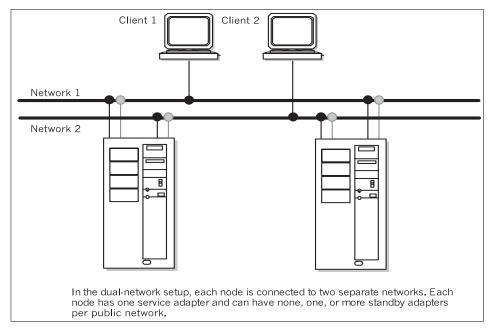
Figure 2-10 Dual-network setup
