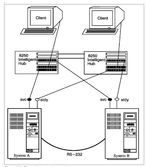
Figure 3-3 Connecting networks to a hub
