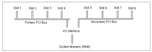
Figure 3-2 Multiple primary PCI buses
