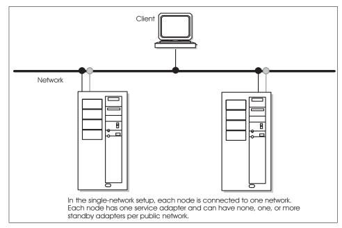
Figure 2-9 Single-network setup
