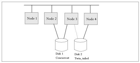
Figure 9-6 CVSD and RSVD I/O example
