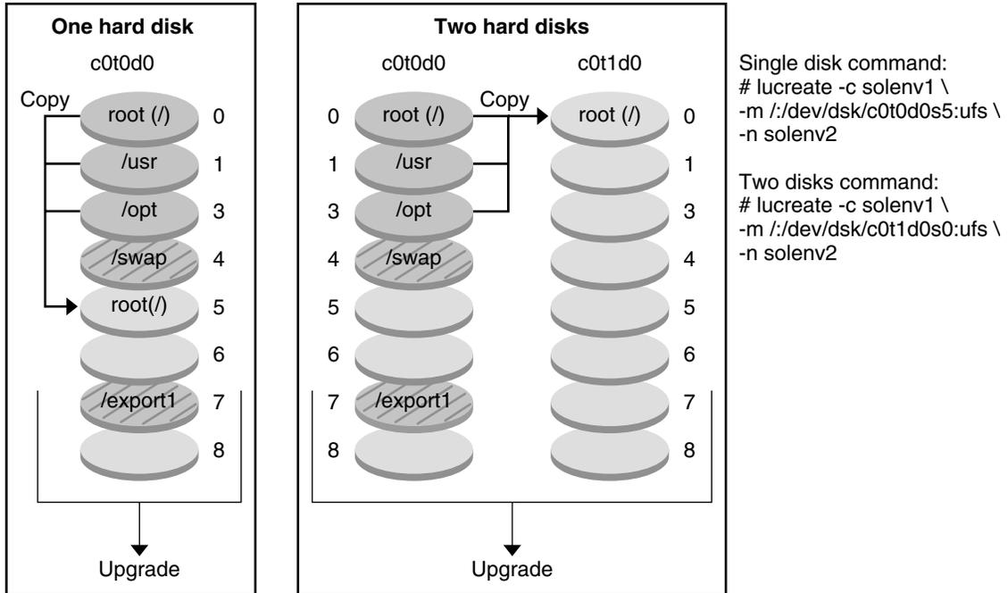
**FIGURE 6-4** Creating an Inactive Boot Environment – Merging File Systems
