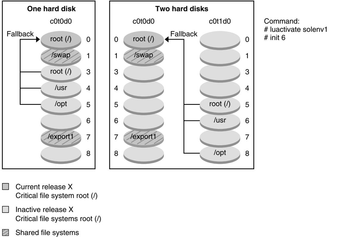
FIGURE 6-11 Fallback to the Original Boot Environment
