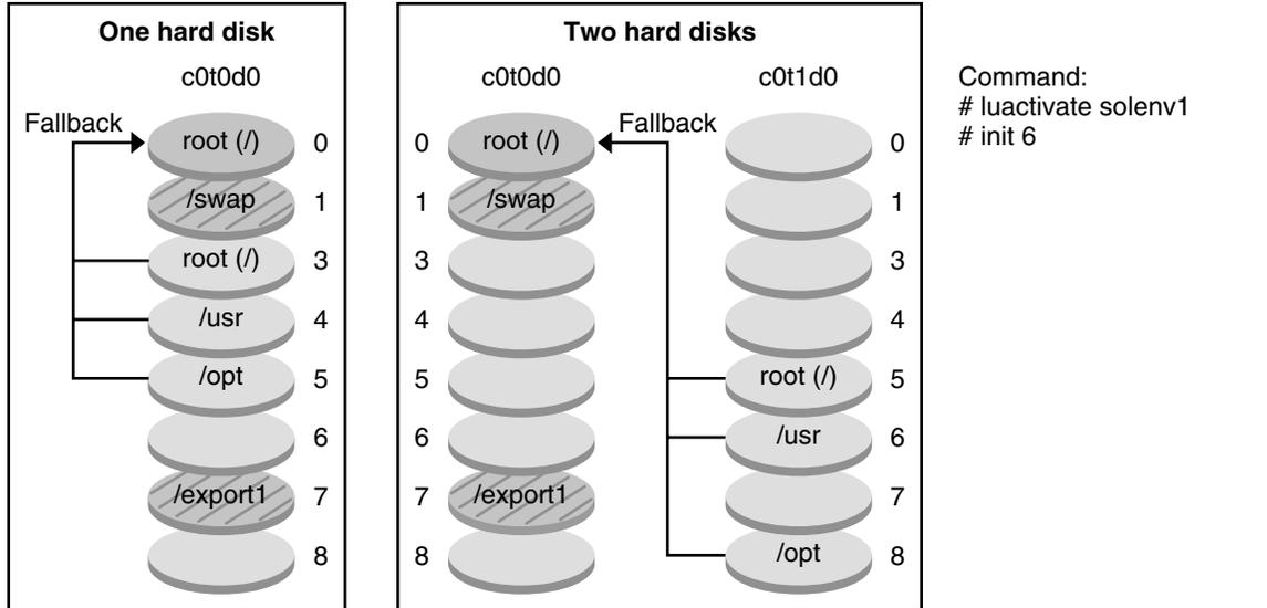
FIGURE 6-11 Fallback to the Original Boot Environment
