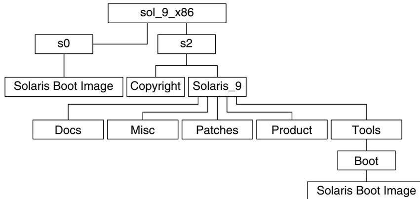
**FIGURE 38-8** x86: Solaris 9 Software 1 of 2 *x86 Platform Edition CD*
