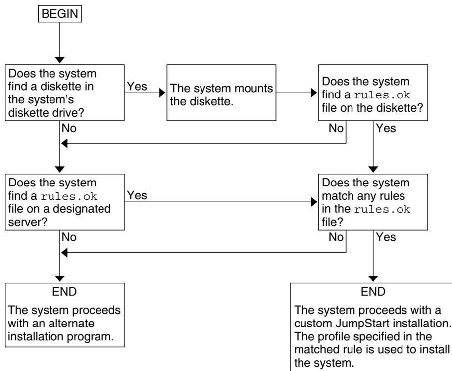
**FIGURE 22-3** What Happens During a Custom JumpStart Installation
