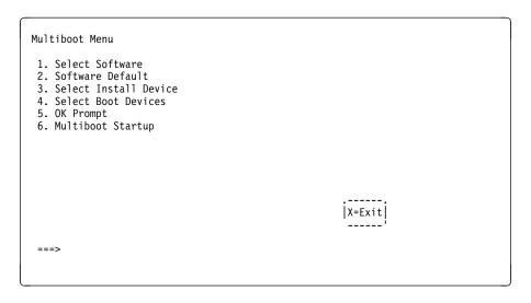
Figure 7-4. Text-based System Management Services - Multiboot Menu
