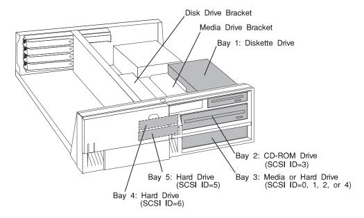
Use the following SCSI cable routing table to ensure all cables are reattached correctly.
