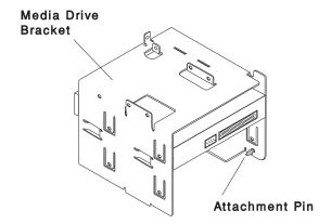
4. Remove the screw which secures the media drive bracket to the side of the chassis, then remove the media drive bracket assembly.
