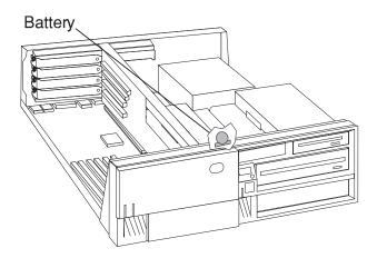
c. Remove the battery as shown.
