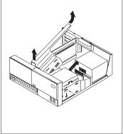
4. Disconnect all cables attached to the riser card.
