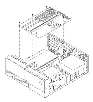
8. Lift the system board out of the system unit.
