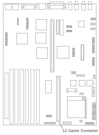
3. Gently pull upward on the L2 cache card, remove it from the system unit, and store it in a safe place.
