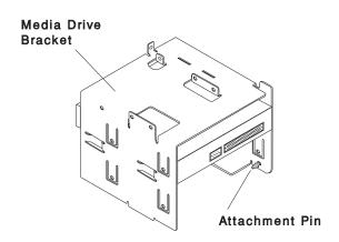
5. Remove the screw which secures the media drive bracket to the side of the chassis, then slide the media drive bracket assembly to the rear of the system unit.
