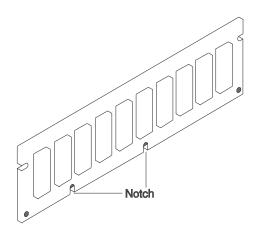
2. Insert the memory module into the next unused memory connector. Push down on the memory module until the latch tabs lock the memory module into the connector. (Do not attempt to move the latch tabs yourself. They lock automatically when you have fully inserted the memory module.)
