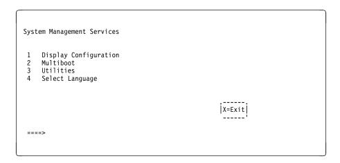
Figure 7-2. Text-based System Management Services - Main Menu (Model 150)
