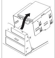
5. Remove the screws which secure the media or disk drive within the media drive bracket.
