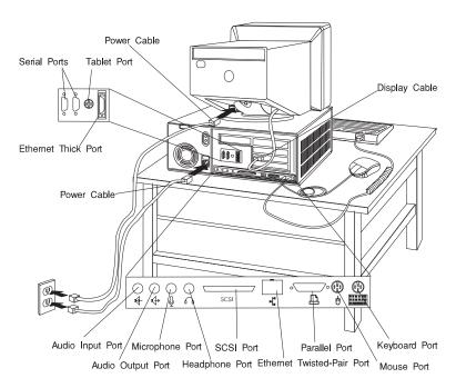
3. If you have a modem or fax machine attached to the system unit, reconnect the telephone line to the system unit and the wall outlet.
