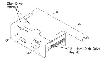
Replacement: To replace, perform the removal steps in the reverse order. Be sure to match the SCSI addresses of the replacement disk drives with those of the removed disk drives. Recommended SCSI addresses are shown in the illustration on page 8-13
