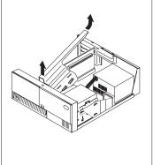
2. Remove the media fan assembly and disconnect the media fan cable.
