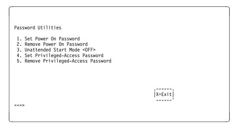
Figure 7-10. Text-based System Management Services - Password Menu
