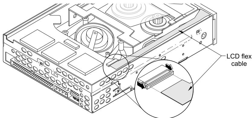
**Figure 8** Loosening the tab on the LCD flex cable connector
