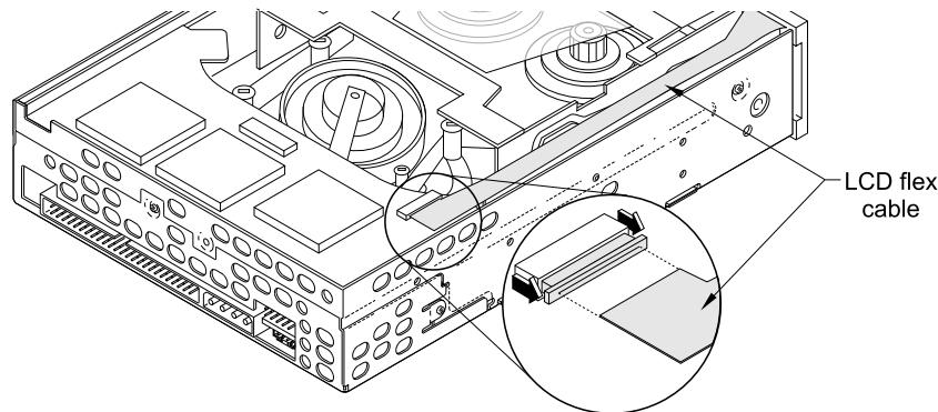
**Figure 2** Loosening the LCD flex cable connector
