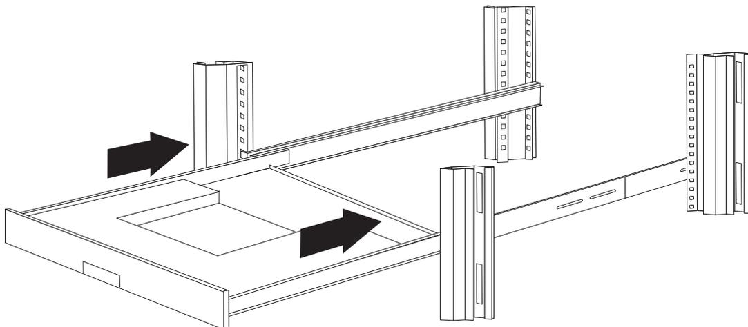
9. Slide the tray in and out several times to check for smooth operation.
