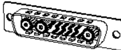
Figure B - Male 13W3 connection on the cable's end.
