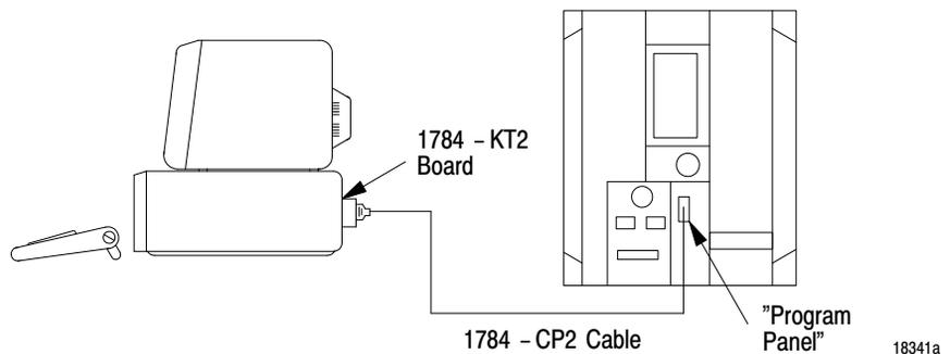
2. Connect the other end of the 1784-CP2 cable into the PROGRAM PANEL connector on the PLC-2.
