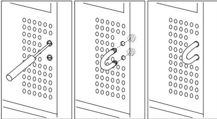
4. If you have completed installing the U-bolt and do not want to install any other internal options, replace the server side cover and reconnect all external cables and power cords. (See “Completing the installation” on page 77 if you need additional information.)
