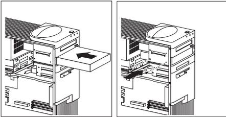
4. Attach the cables to the drive. See "ISA and PCI adapters" on page 61 for an illustration that shows the locations of the connectors on the riser card.
