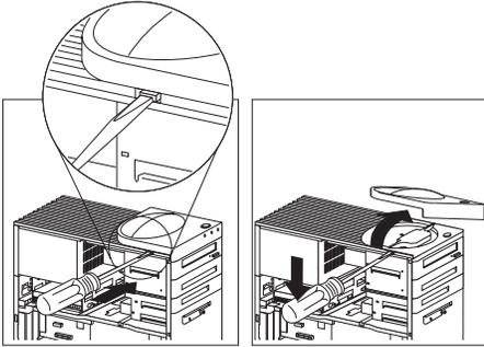
3. Remove the top-handle screw and the screw from the drive-support bracket that holds the upper drive cage in place. Then, move the drive cage towards the power supply until it stops, and lift it out of the server.
