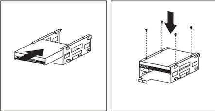
5. If you are installing a drive in bay 6, turn the drive upside down before you slide it into the bay. This ensures that the drive connector will align with and attach properly to the cable connector.
