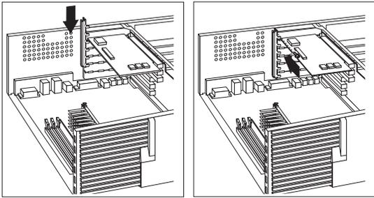
9. If you installed a network adapter that uses Wake on LAN or Alert on LAN, attach the cable from the riser card to the adapter. See "ISA and PCI adapters" on page 61 to locate the Wake on LAN or Alert on LAN connector. If you installed a modem and want to use Modem Wakeup, see "ISA and PCI adapters" on page 61 to locate the Modem Wakeup connector on the riser card.
