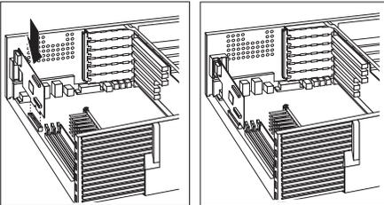
4. If necessary, connect any internal cables to the adapter. Refer to the documentation that comes with the option.
