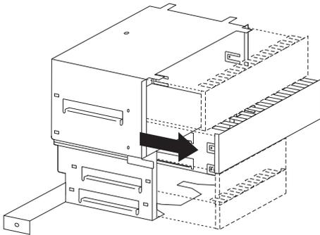
2. Touch the static-protective package containing the new drive to any *unpainted* metal surface; then, remove the drive from it.
