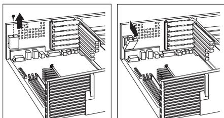
3. Install the AGP adapter. The following illustration shows the installation of an AGP adapter. Note that the connector for external devices on the AGP adapter is accessible through the slot on the server wall.
