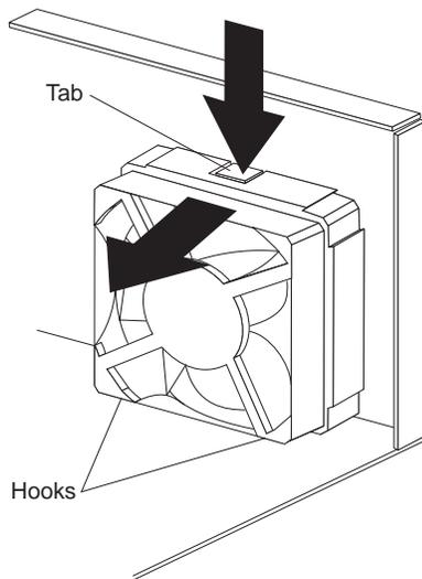
5. Replace the front fan by aligning the two hooks on the bottom of the front fan assembly with the slots on the server wall.
