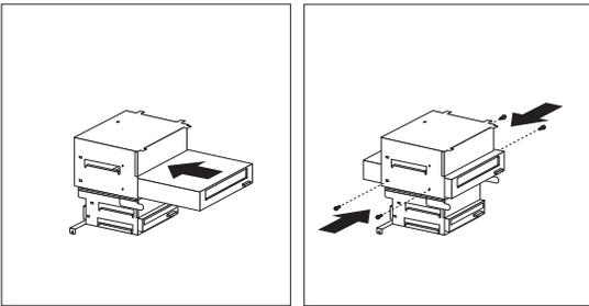
4. Insert the drive cage and slide it to the right until it stops at the front of the server; be sure that the screw holes in the drive cage are aligned with the screw holes in the support bracket.
