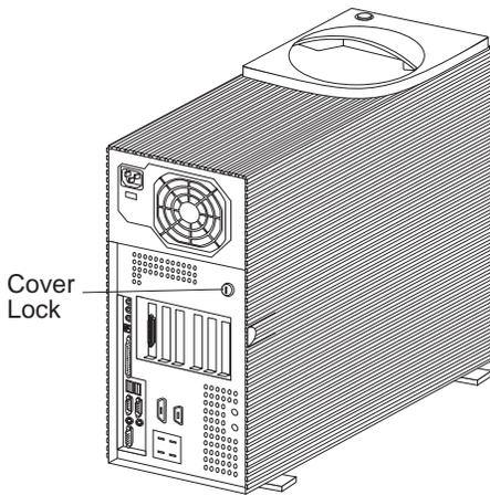
9. Remove the side cover by pulling out on the cover-release tab at the rear of the side cover. Then, slide the cover toward the front of the server and lift it off.
