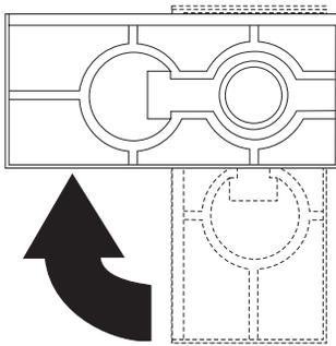
When you need to access the inside of the server to install options, you might find it easier to place the server on its side, so that the system board is facing you. If you do so, rotate the feet in towards the server, so that they do not detach due to the weight of the server.
