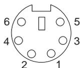
Table 8 shows the pin-number assignments for the keyboard and auxiliary-device port connectors.
