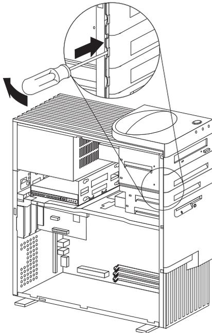
2. If knockouts are present in the drive bay opening, twist them with a screwdriver or pliers to remove. The following illustration shows the type of knockout in bays 2 and 3.
