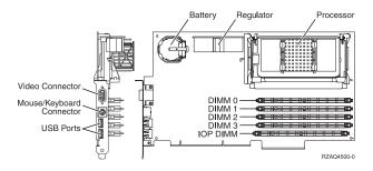
Figure 10. Locations of DIMM 0, DIMM 1, DIMM 2 and DIMM 3 on 2890 Integrated xSeries Server (IXS) card.
