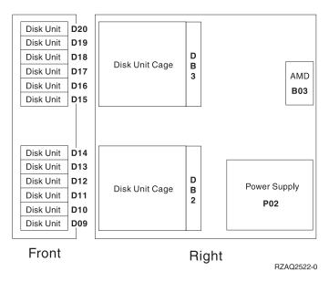
Figure 28. Model 270 FC 7104 System Unit Expansion
