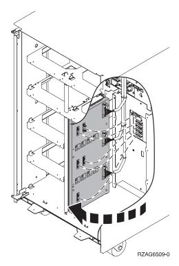
7. Remove the cables from the rear of the DASD board assembly and note their locations.
