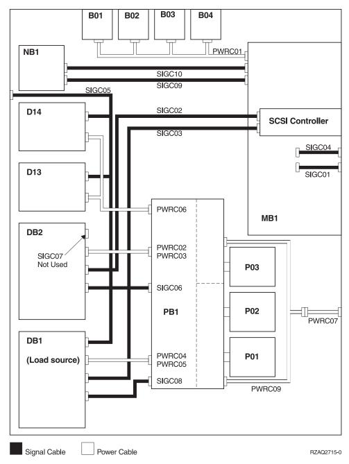
Figure 46. Model 820 - Single Line Cord Power and Signal Cables (Dual Line Cord Enabled)
