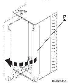
7. Install the power supply by reversing the removal procedure. After exchanging an item, go to "Verifying the Repair" on page 830.
