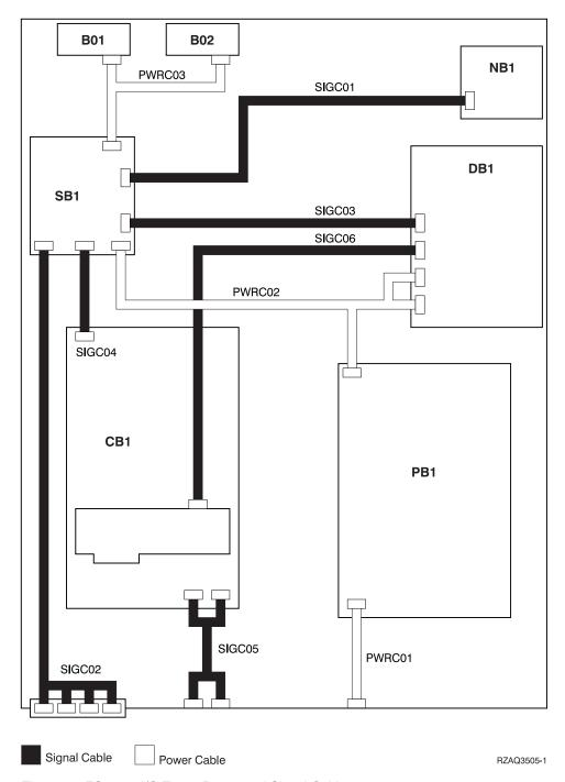
Figure 50. FC 5075 I/O Tower Power and Signal Cables
