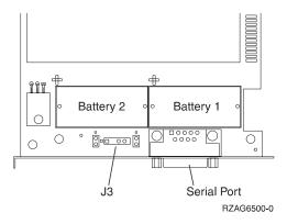
Figure 21. Battery Locations on the 4758 PCI Cryptographic Coprocessor
