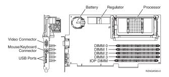
Figure 9. Locations of DIMM 0, DIMM 1, DIMM 2 and DIMM 3 on 2890 Integrated xSeries Server (IXS) card.
