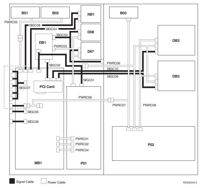
Figure 44. Model 270 (with System Unit Expansion) Power and Signal Cables
