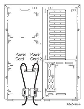
Figure 31. Dual Line Cord Drawing for Model 820 System
