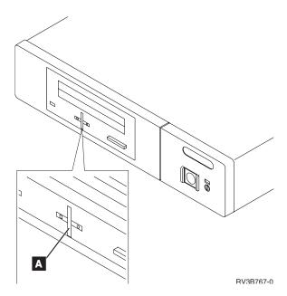
3. Insert a solid metal rod (like a bristol wrench) into the manual tape cartridge unload hole and push in until it stops and the arm appears.
