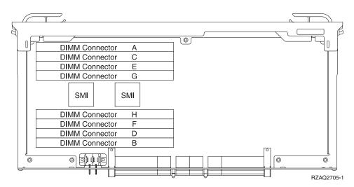
Figure 41. Processor Card with DIMM memory
