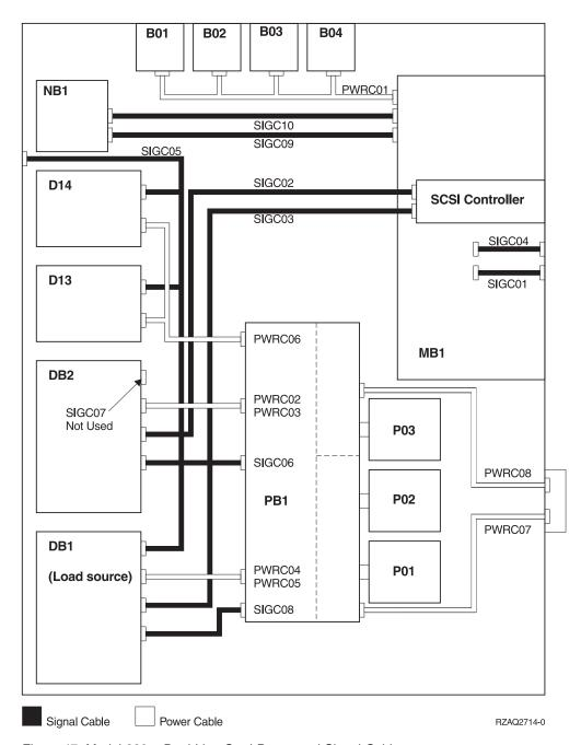
Figure 47. Model 820 - Dual Line Cord Power and Signal Cables
