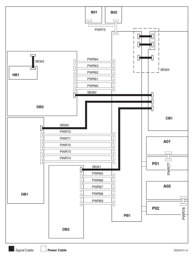
Figure 49. FC 5074 I/O Tower – Dual Line Cord Power and Signal Cables
