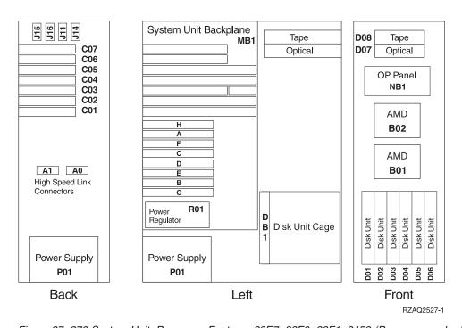
Figure 27. 270 System Unit, Processor Features 23E7, 23F0, 23F1, 2452 (Processor embedded on backplane)
