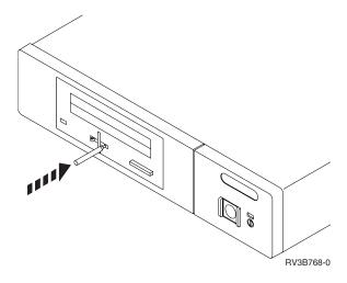
4. Pull the arm out until it stops. Insert the solid metal rod into the hole of the arm and pull out until the tape cartridge comes out.
