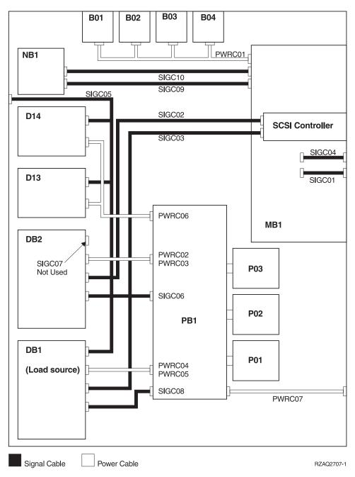
Figure 45. Model 820 - Single Line Cord Power and Signal Cables (Non-Dual Line Cord Enabled)
