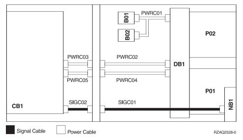
Figure 51. FC 5078, 0578 I/O Tower Power and Signal Cables
