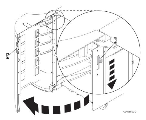
Figure 15. Rear Cover - Removal
