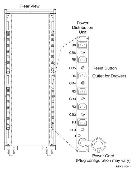
Figure 39. Locations for the Power Distribution Unit (PDU)
