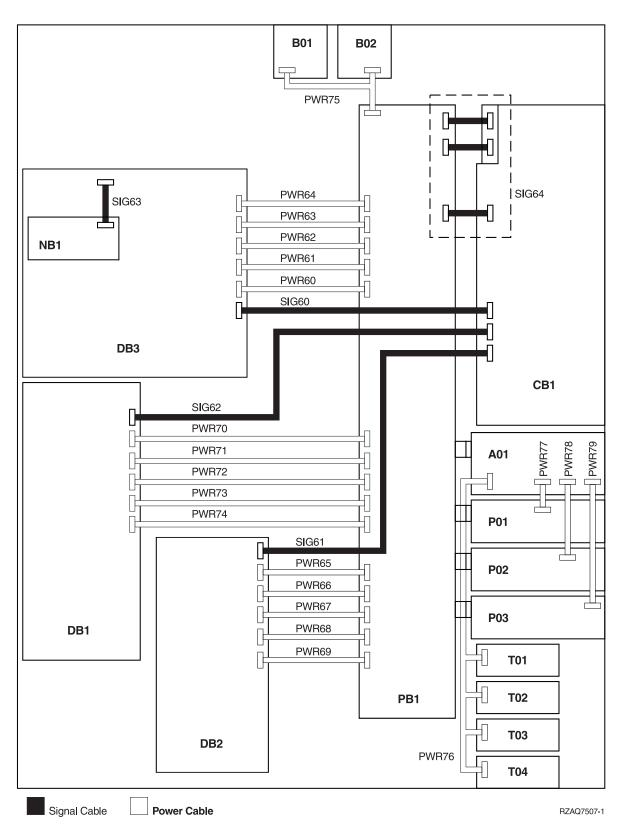
Figure 48. FC 5074 I/O Tower - Single Line Cord Power and Signal Cables
