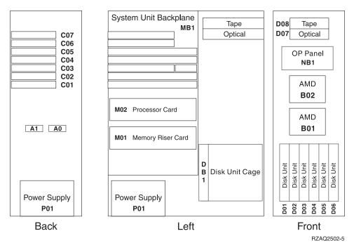
Figure 26. 270 System Unit, Processor Features 22A7, 22A8, 22AA, 22AB, 23F4, 23F5, 2423, 2424, 2454
