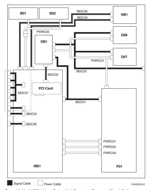
Figure 43. Model 270 (without System Unit Expansion) Power and Signal Cables
