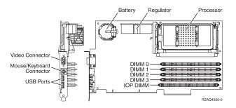
Figure 13. Locations of DIMM 0, DIMM 1, DIMM 2 and DIMM 3 on 2890 Integrated xSeries Server (IXS) card.
