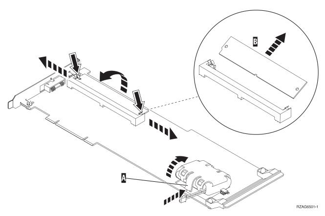
Figure 20. Cache Battery Pack and Cache Directory Card for Type 2748, 2763, 2778
