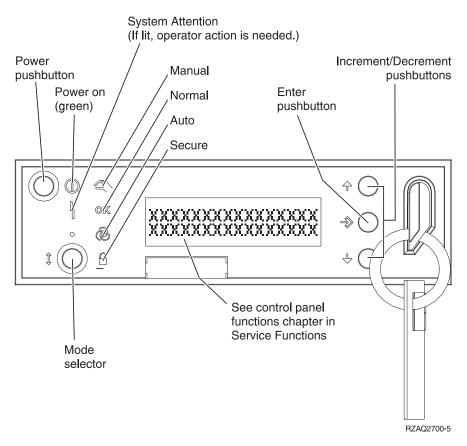
Figure 6. Model 820 Control Panel layout with keystick
