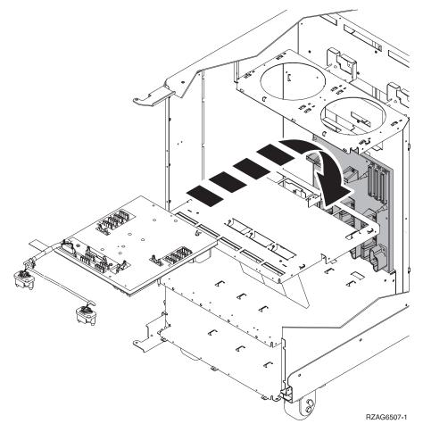
7. Install the power distribution backplane by reversing the removal procedure. After exchanging an item, go to "Verifying the Repair" on page 830.
