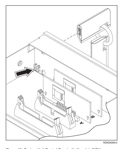
Figure 18. System Unit Control Panel with Keystick (NB1)
