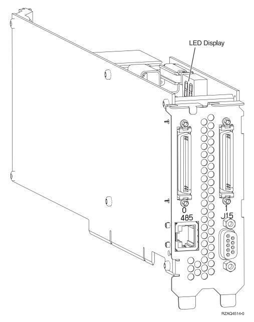
Figure 38. Locations for xSeries Adapter Card
