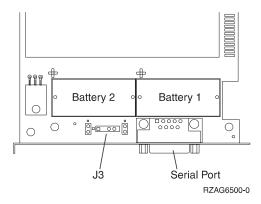
Figure 22. Battery Locations on the 4758 PCI Cryptographic Coprocessor
