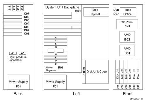
Figure 25. 270 System Unit, Processor Features 22A2, 22A4, 22A5, 2301, 2302, 2422 (Processor embedded on backplane)
