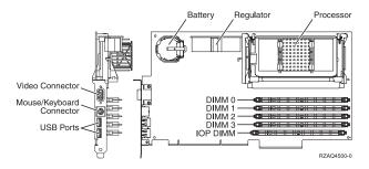
Figure 11. Locations of DIMM 0, DIMM 1, DIMM 2 and DIMM 3 on 2890 Integrated xSeries Server (IXS) card.
