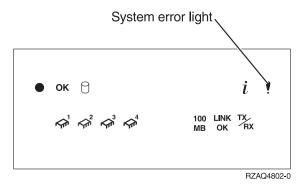
Figure 7. Integrated xSeries Server (IXS) - Control Panel
