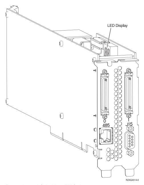
Figure 19. Integrated xSeries Adapter (IXA) Card
