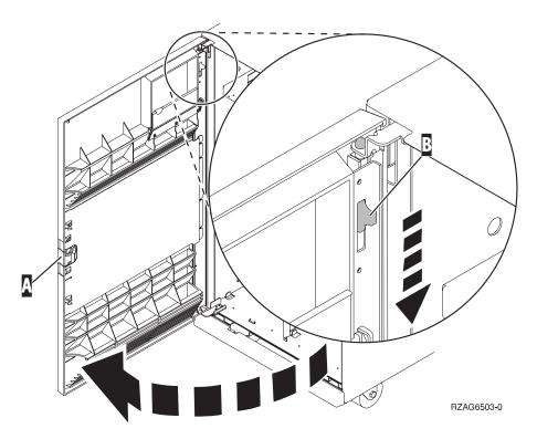
Figure 14. Front Cover - Removal
