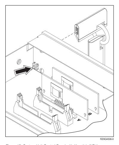
Figure 17. System Unit Control Panel with Keystick (NB1)
