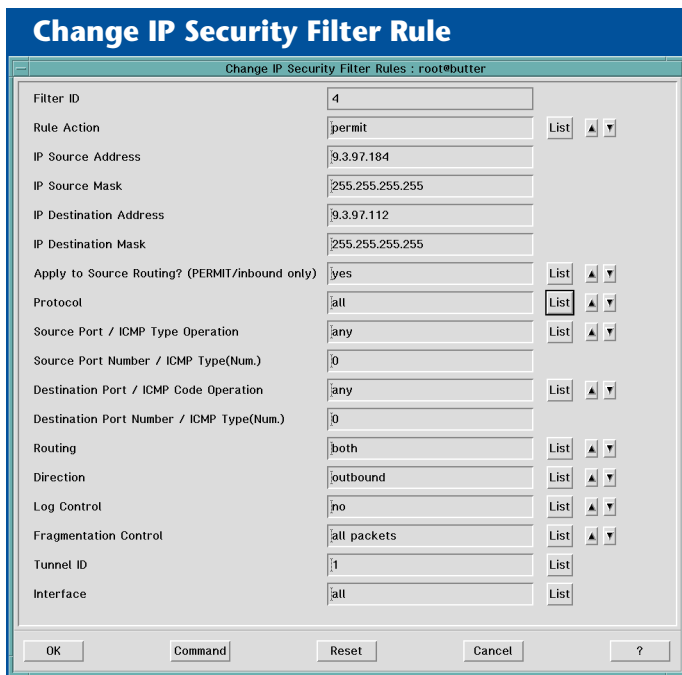
Figure 7. Filter rule for change IP security
